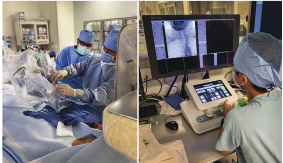
Left: Sterile Corpath GRX patient-side robotic system during setup. Right: Lead-shielded remote Corpath GRX control station during cerebral angiography procedure.
